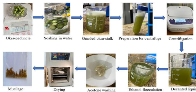
Centrifuge-assisted mucilage extraction from okra peduncle
