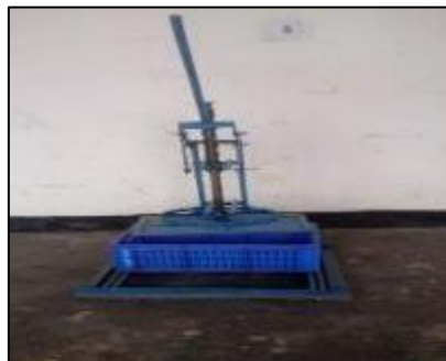
Manual mushroom bed compaction unit
