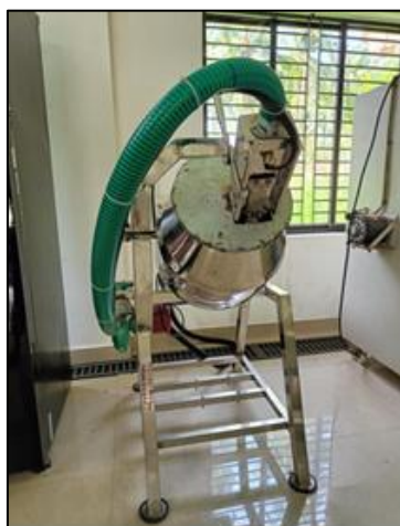
Rotary Dryer for drying and flavour coating of coconut chips
