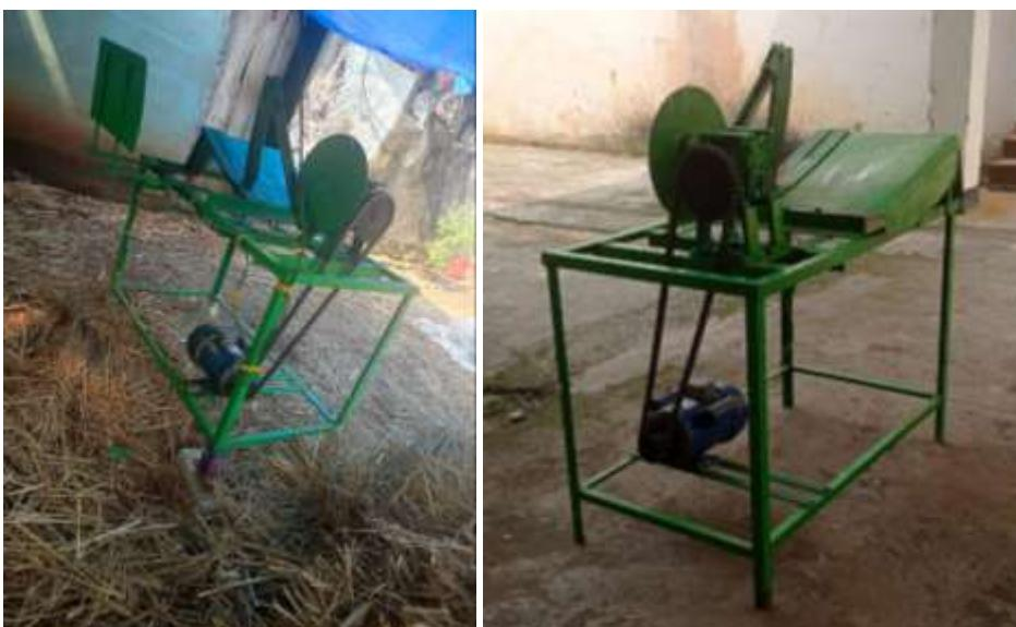
With an impressive capacity of 800 bundles per hour and a low power requirement of 0.375 kW, it is energy-efficient. Priced at Rs. 50,000, it offers an economical solution with a production cost of Rs. 0.30 per bundle. Requiring only one operator, the machine streamlines straw processing, making it ideal for large-scale farming while improving productivity and reducing manual drudgery in mushroom cultivation.
