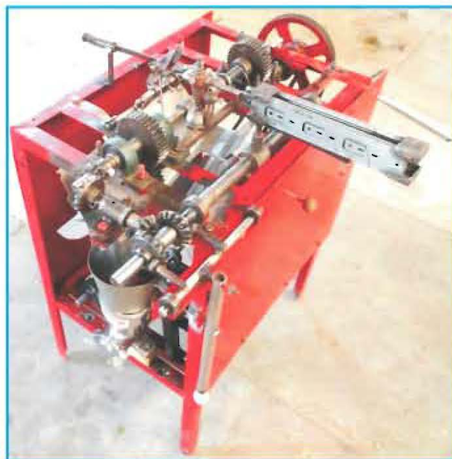
Side view of the developed peeler cum juice extractor
