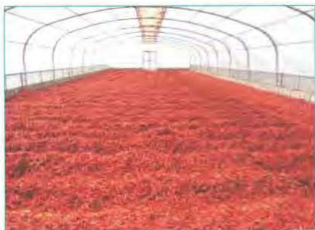
Modified ANGRAU polyhouse solar dryer for chillies
