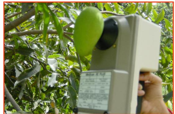
any colorimeter. Method is nondestructive and easy to use at any place.
