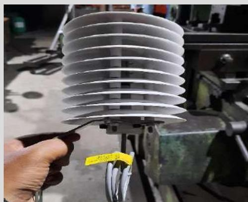
low cost solar radiation shield system
