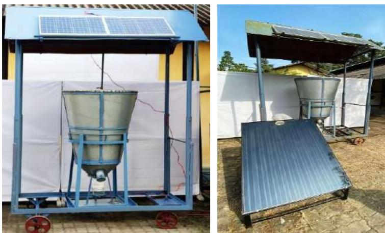
*Storage structure with air solar air blower - Solar air heater*
