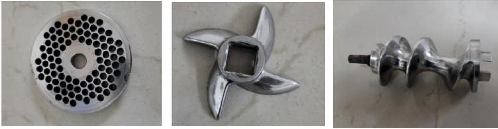
Figure 6. Different parts of meat mincer: plate, blade, and barrel.
