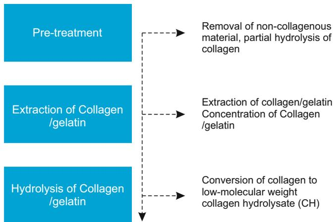
Figure 3. Basic steps for production of collagen hydrolysate.
