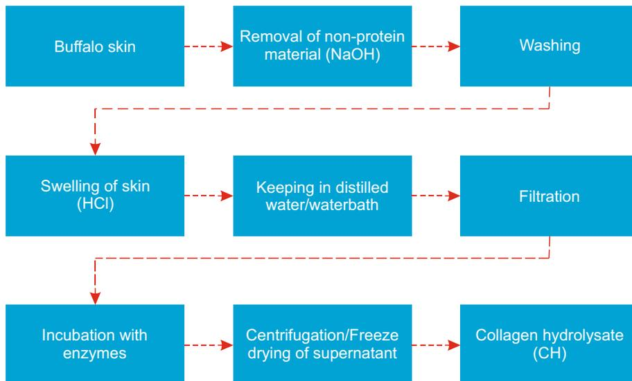
**Figure 5. Enzymatic method for production of collagen hydrolysate.**
