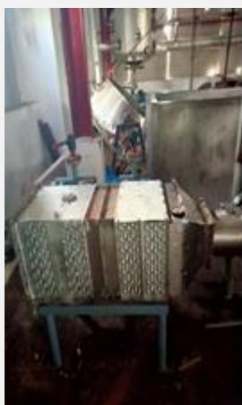
**Dehumidifier for removal of moisture from granular jaggery**
