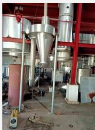
**Pneumatic aspiration system for conveyance of granular jaggery**
