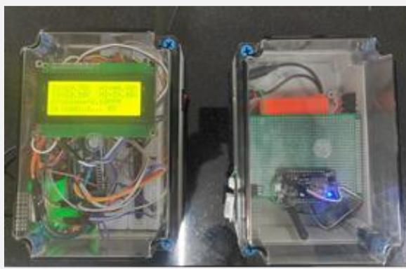
Modified prototype of the sensor-based system (Cluster node in left and sensor node in right)
