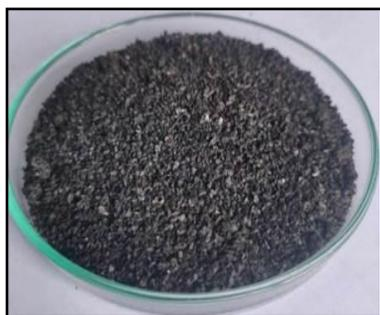
Pyrolysed carbon @ 300°C
