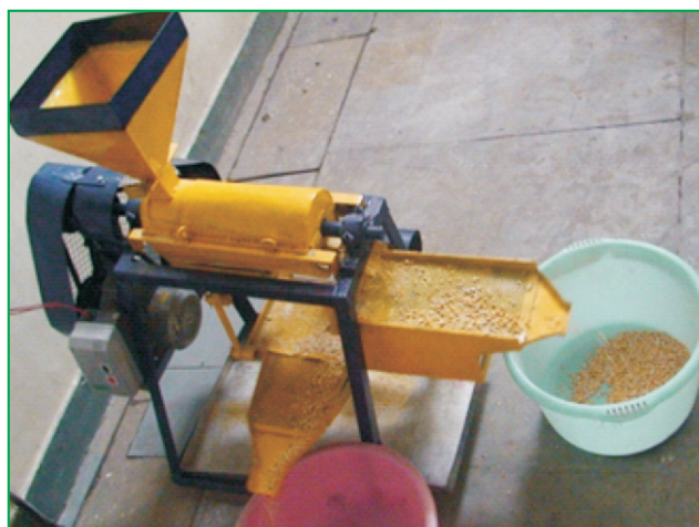
Fig. 38. A small capacity maize degermer, fabricated at CIPHET, Ludhiana
