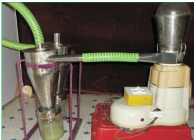
Fig. 84. Pilot plant for tender wheat shoot powder
