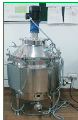
Fig. 9. Integrated pilot plant for pretreatment, hydrolysis and fermentation for production of value added products from crop residues
