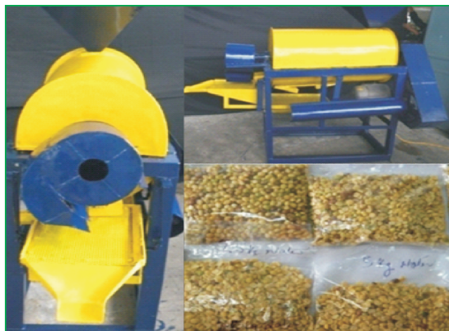
Fig. 34. CIPHET Developed Single Feed Composite Pigeon Pea Mini Dhal Mill
