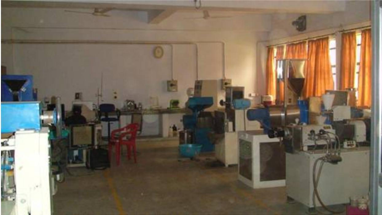
The laboratory has different processing equipment for bakery and extruded products. Different types of extruders such as low cost single screw collet, rotary head and double screw extruders are available. Apart from above the laboratory is also equipped with wet and dry grinding systems, aonla pricking machine, juice maker, flour sifter, pasta making machine etc.
