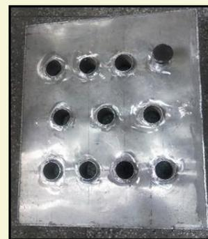
Fig 2. PCM chamber for thermal storage
