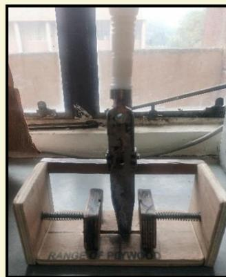
Fig 1. Hand tool mango stone decorticator
