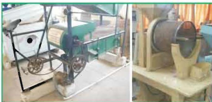
Fig. 8: Pedal cum power operated air screen grain cleaner cum grader
