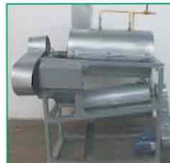
An integrated machine for breaking of bael/wood apple
